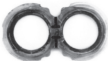
Wearplate showing the effects of overheating
