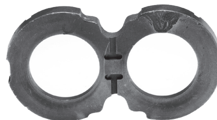
Wearplate showing pitting from cavitation
