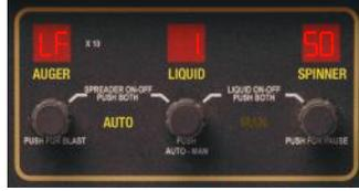
(up & down) operation when those keypads are pressed. Set a value on the Spinner display and push the Spinner knob to enter.
