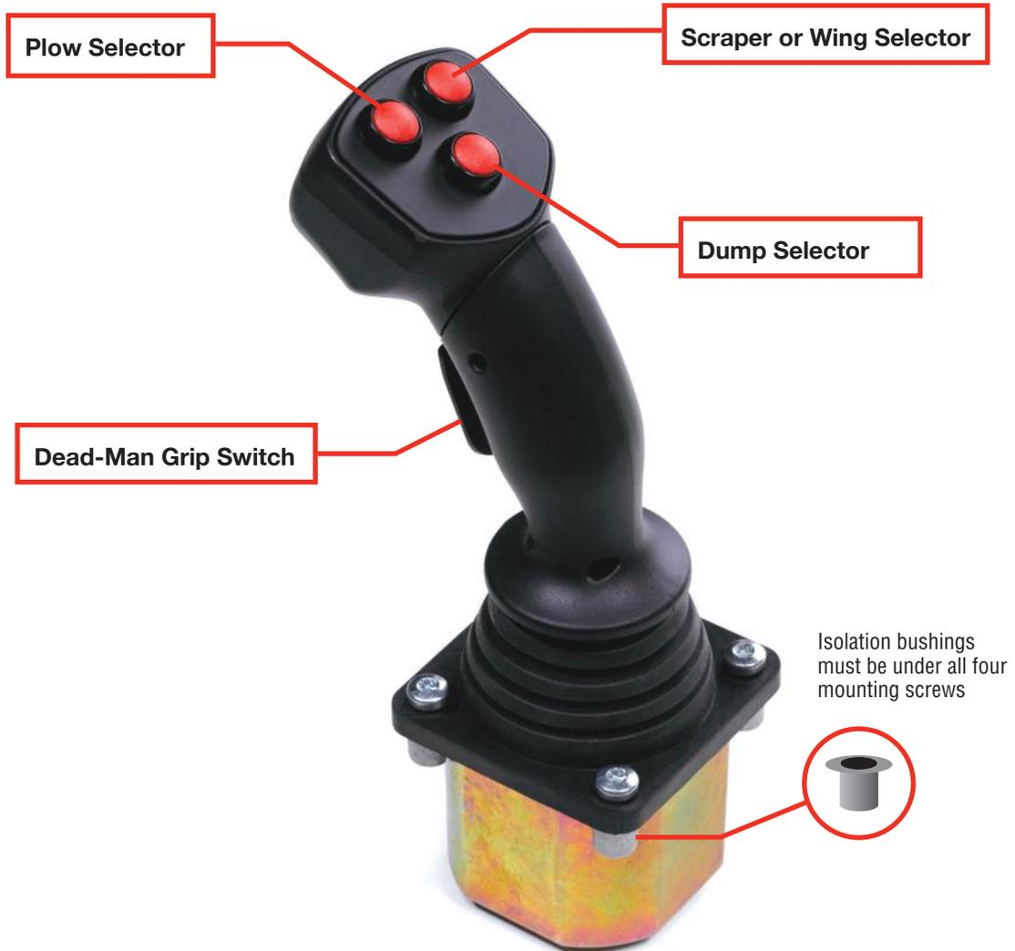
The Dead-Man Switch must be depressed BEFORE moving the joystick from center and MUST be held throughout the operation. If released, the joystick must be returned to center to re-activate the Dead-Man switch.
