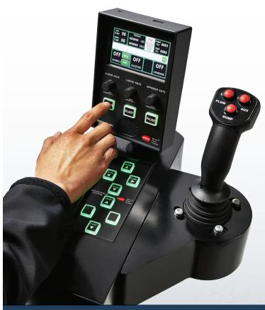
Systems like Muncie Power Products' Advantage+ snow and ice control system combine this type of real-time, Wi-Fi support with advanced GPS data logging. The data-log report software provides organized reports with filtering capabilities for reviewing information such as truck routes, spreader rates, totals and more. This ability to review system operation allows the supervisor to ensure the truck is operating at peak efficiency.
