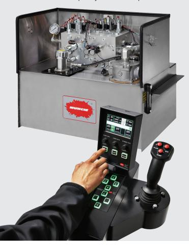
Sturdy and durable stainless or powder-coated enclosures come standard as part of the system's rugged design. Last - but not least - one, centralized location on the truck houses the hydraulic valves, return line filter, clean out, electrical modules and more. This one, centralized location makes servicing the system simple and easy.
